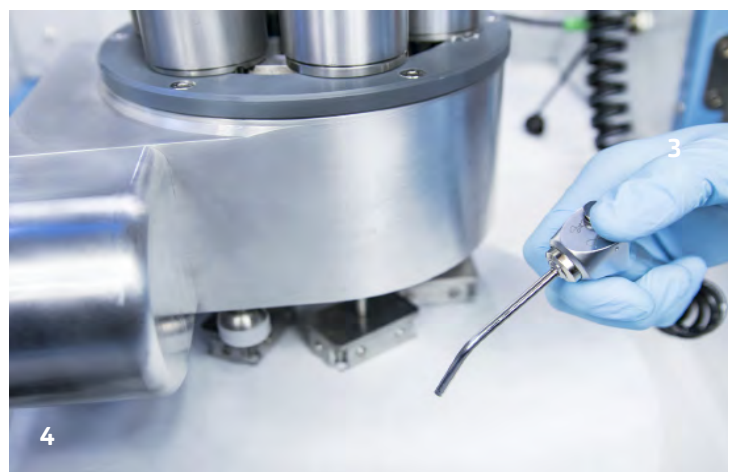
1: PM6 Precision Lapping & Polishing System 2: Metered abrasive feed unit via peristaltic pumps 3: Bluetooth enabled automatic plate flatness monitor 4: Integrated sample cleaning with de-ionised water and nitrogen gun
