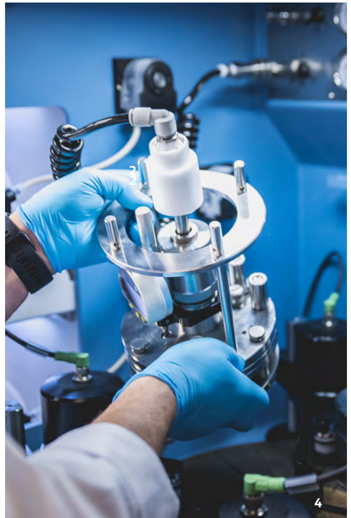
1: LP70 Precision Lapping & Polishing System 2: Process conditions controlled via the Graphical User Interface 3: Bluetooth enabled automatic plate flatness monitor 4: Four workstations each with a wafer process capacity of 100mm/4"
