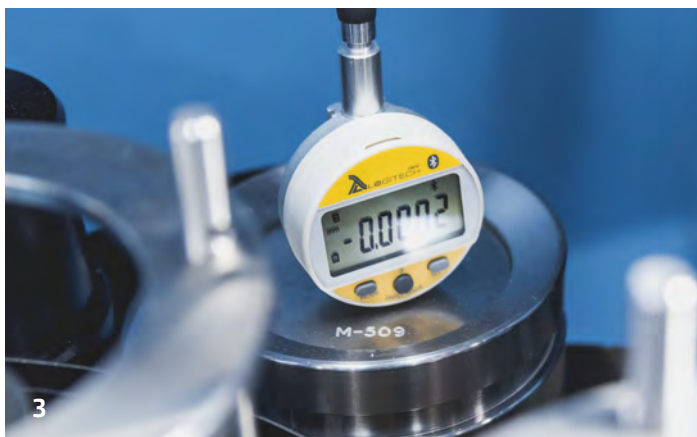
1: LP70 Precision Lapping & Polishing System 2: Process conditions controlled via the Graphical User Interface 3: Bluetooth enabled automatic plate flatness monitor 4: Four workstations each with a wafer process capacity of 100mm/4"
