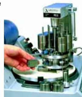
The WG2 polishing system - a rapid and economical method for polishing geological samples.
