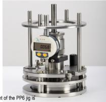
Fine adjustment of the PP6 jig is easy using the Sample Loading Gauge.
