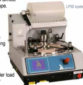
Lapping plate flatness control improves the quality and repeatability of the thin sections produced. It is of tremendous advantage to the operator - freeing a large amount of the time which would be spent on machine supervision for other tasks, such as analysis, and improving the overall productivity of the thin section production system.
